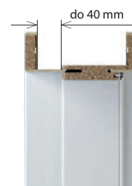
maximum door frame with a wider tongue optional at an extra charge
