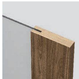
glass - door panel joint non-rebated door
