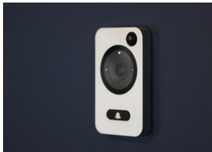
Electronic spy hole with a doorbell, memory card, and infrared photo camera with motion detection
