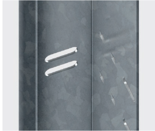
Double fixing holes – holes in the opening frame (special holes provided in the frame for installing anchors). This is convenient whenever fitting problems arise, e.g. when the drill hits a rebar while holes are being drilled.
