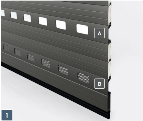
1 Door curtain – made of aluminium profiles 100 [mm] high and 25 [mm] thick infilled with freon-free polyurethane foam. (A) – glazed single-wall aluminium profile, (B) – ventilated single-wall aluminium profile.
