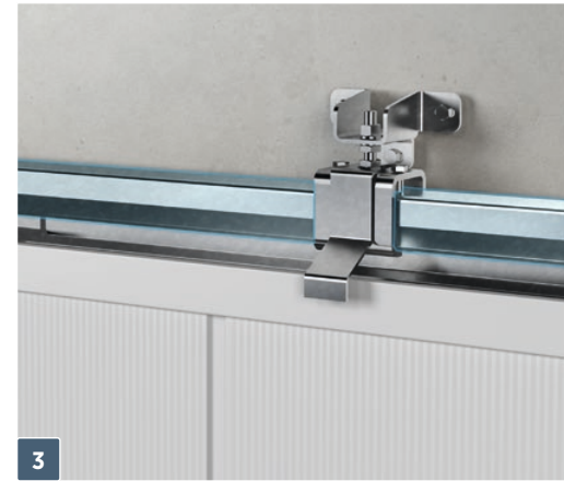
3 Running track – made of a hot-dip galvanized steel channel section. The running track is fixed to holders enabling 2-plane adjustment. The ends of the track are fitted with rubber bumpers that prevent the leaf from sliding out.
