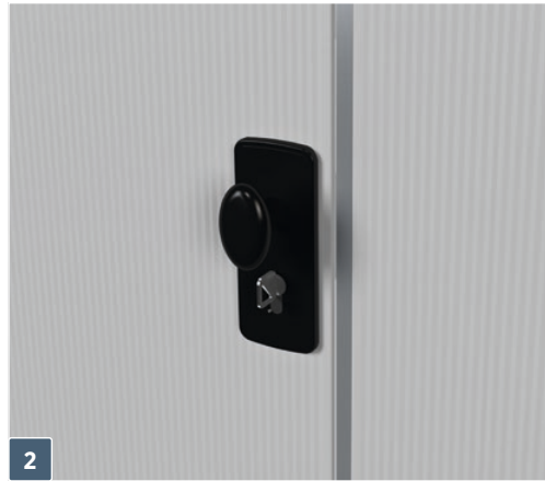
2 Lock – both active and passive leafs are bolted in two points (in the top and bottom section). The active leaf is fitted with a plastic handle from the outside and from the inside, a single-side lock cylinder accessible from the outside, and a lock operated with a latch from the inside.
